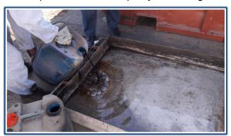
4.4 A strip of hydrocarbon detector was used to check the presence of oil in the; the result was positive.
