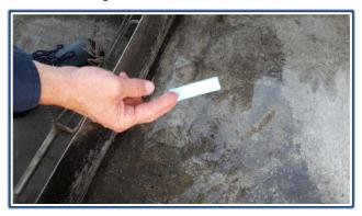
4.3 Oil was poured onto the drip tray containing water.
